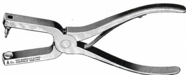
TOECAP PUNCH PLYER, Jaw 2 inches long.
