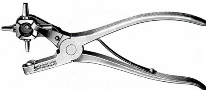
SOLID REVOLVING PUNCH PLYER, Four Bits.
