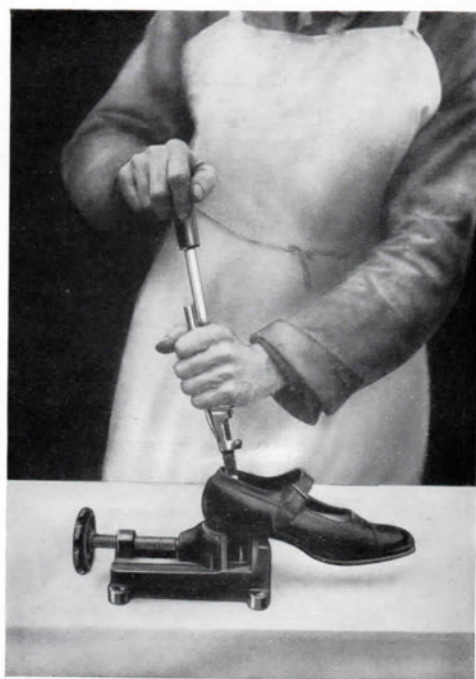
TUBULAR NAILER, with feed tube and hand rest.
